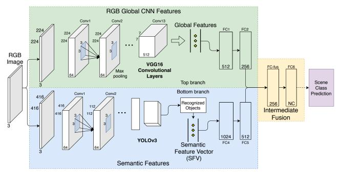
Fig. 2. An overview of the proposed  $GSF^2App$  (in FC6, NC represents the output number of classes). The top branch (green) uses the VGG16 network to extract global features. The bottom branch (blue) uses the YOLOv3 model to recognize the objects present in the scene, which are encoded into a Semantic Feature Vector. Both branches converge in two fully connected layers (yellow).
