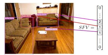
Fig. 3. Example of how YOLOv3's output object class predictions are encoded into a Semantic Feature Vector. Sample indoor scene image taken from the NYU Depth Dataset V2 [8].
