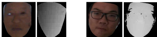
Figure 5: Comparison between RGB and depth images of a print attack (left) and a bonafide face (right). Note that the depth images aren't of great quality, not being able to capture the eyes cut out of the print attack and not giving much detail to the bonafide case, but being possible to notice the differences. Images selected from the CASIA-SURF dataset (Zhang et al., 2019b).
