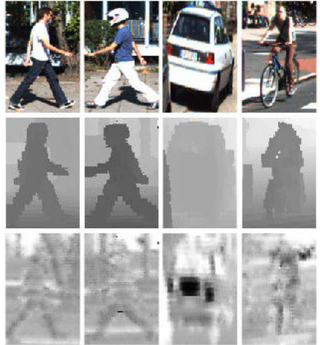
Fig. 3. In the first row we have examples of pedestrians and non-pedestrians from the monocular camera. The last two rows show the corresponding depth and reflectance maps generated from LIDAR data.
