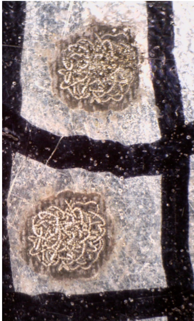
Figure 8. Laser mark with (path) A repeated in two different marks. Top mark is A1 and bottom mark is A2
