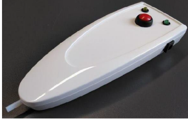
Figure 4. Dispersant tool (prototype version) used to deposit a certain amount of diamond particles on the metal surface. New automatic and more practical dispersant tools were designed and are being produced.
