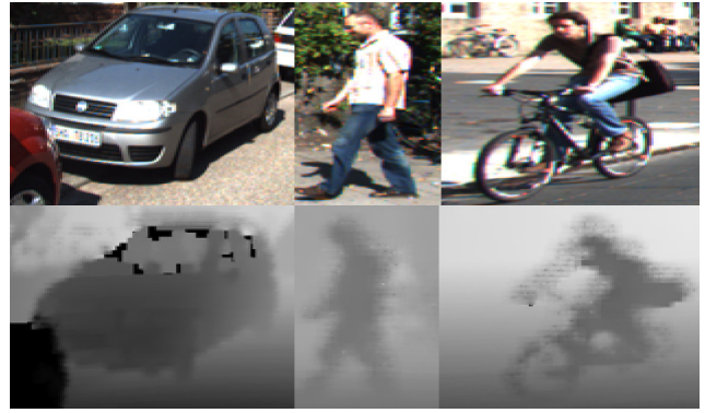
Fig. 4: Labeled car, pedestrian, and cyclist examples on RGB (colour images) and DM representation.
