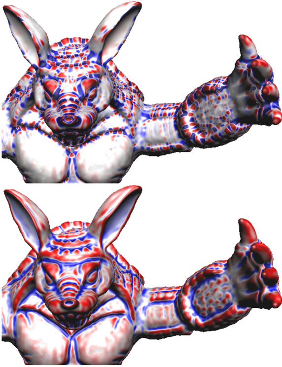
Fig. 1. Gaussian and mean curvatures of the smooth Armadillo model.
