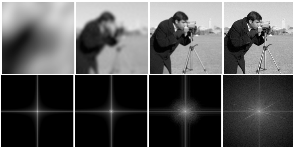
Fig. 18. Cameraman - reconstructed multiresolution levels 1, 3, 5 and 7 and corresponding Fourier spectra.
