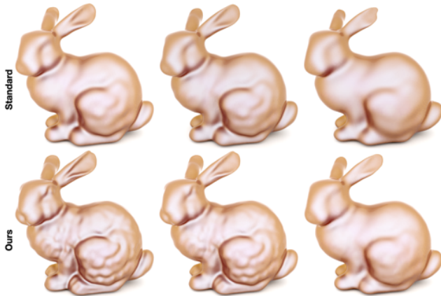
Figure 13. Network initialization comparison. Line 1 shows the results of using the initialization is given in [33] and Line 2 considers the proposed initialization. Notice how the new network initialization results in a model that can represent higher frequencies, as shown by the increased surface details in Line 2.
