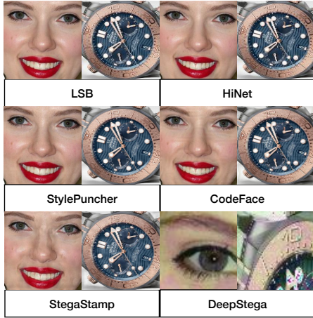
Figure 5: Examples of steganography models that encode a hidden message into image’s ROI. The size of DeepStega’s input and output is 64 \times 64 \times 3 , smaller than other models. Therefore, for a fair comparison, we use a smaller encoding ROI in DeepStega.
