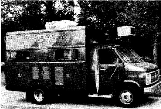
(a) The Navlab's self-driving car [218].
