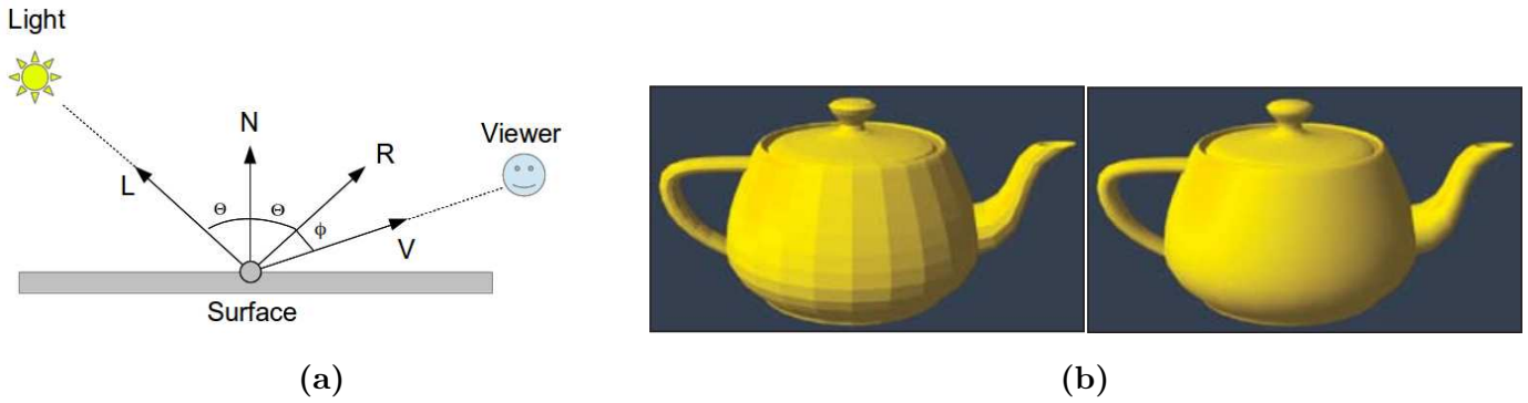
Fig. 2.4: In Fig. (a) it is illustrated the Phong reflection model (the description of the figure is done throughout the section). In Fig. (b) we show an example from [19] for the teapot object when applying different techniques of shading. On the left image a flat shading example and, on the right image, a smooth shading example (Gouraud shading).
