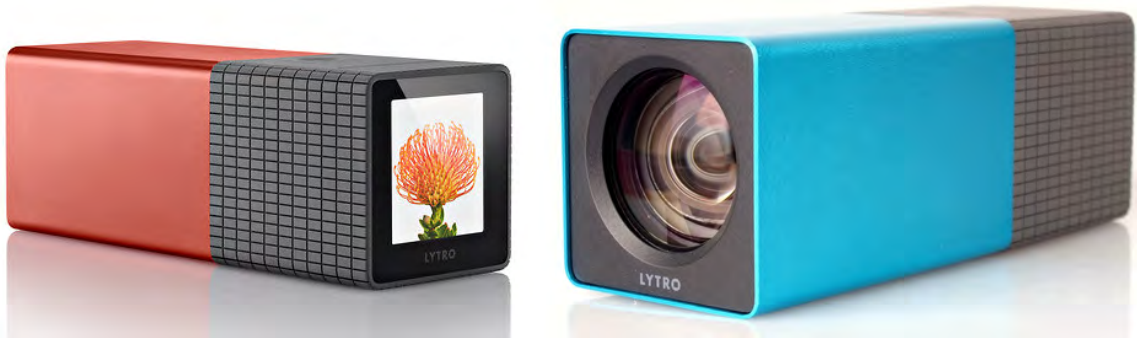
Fig. 2.7: Original Lytro plenoptic camera.
