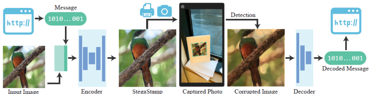
Figure 2.5: Pipeline of the end-to-end solution StegaStamp. First, an encoder network processes the input image and a hidden message. Then the encoded image is printed and captured by a camera. A detection network localizes and rectifies the encoded image before passing it to the decoder network. After the hidden message is recovered and the error corrected, it is possible to follow the hyperlink. Figure from [31].
