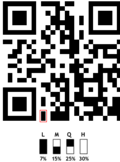
Figure 2.3: Error Correction in a QR code.
