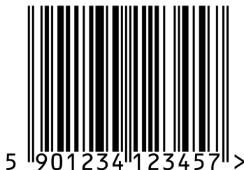
Figure 1.1: The most widely used 1-D Barcode, the EAN-13 [1].
