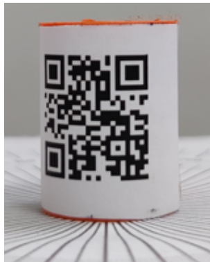
(b) Cylindrical distortion with only tilting.
