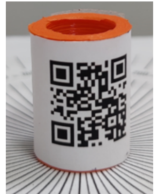
(c) Cylindrical distortion with tilting and sloping
